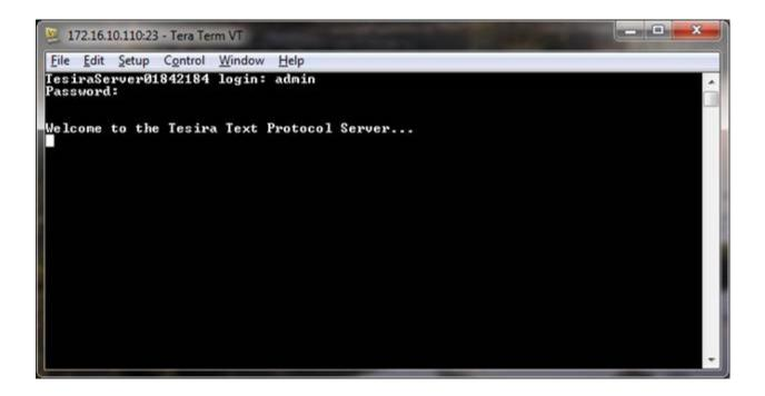
RS-232 Serial connections to the TTP servers also require authentication in protected systems. Making the serial connection and sending a line feed will reveal the login prompt.
