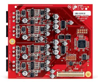
The Tesira<sup>®</sup> EOC-4 is an expander card with 4 analog output channels for use with the Tesira EX-MOD device. The EOC-4 is one of three optional cards that can be mounted in Tesira EX-MOD. Each EOC-4 provides 4 channels of mic or line level audio output. The outputs are electrically balanced and provided on plug-in barrier strip connectors. Software control of each output includes mute, level, signal invert and full-scale output reference.
