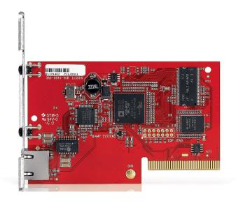
The Tesira® SVC-2 is a modular Voice over Internet Protocol (VoIP) card for use with Tesira SERVER and SERVER-IO devices. The SVC-2 allows a Tesira system to connect directly to IP-based telephone systems. When used in conjunction with Automatic Echo Cancellation processing, Tesira becomes an extraordinarily powerful, flexible and affordable conferencing platform.
