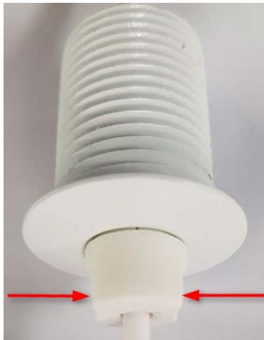
Figure 8 Pinch-points for Microphone Cable Length Adjustment
