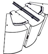
**HAB-BFR38 (1122/1152), HSB-BFR38 (1153):** Horizontal Array Brackets with BalancePoint™ Fly Rails Kit - to array two full-range cabinets with a subwoofer in between
