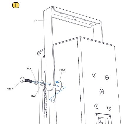
Figure 1. Remove side cabinet bolts and attach yoke to cabinet
