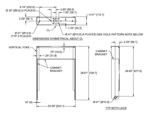
**Hole Pattern Note**: Hole pattern compatible with Chief CMA105 UL listed Ceiling mount adapter plates for use with the manufacturer's respective 1-1/2" NPT rigid pole mounting systems. See manufacturer's websites for mounting details and limitations.
