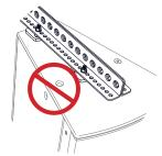
The loudspeaker enclosure must have fasteners in all threaded holes
