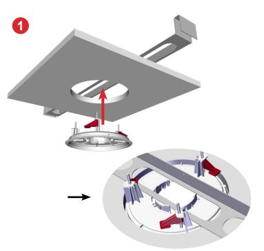
Bracket orientation in tile bridge opening
