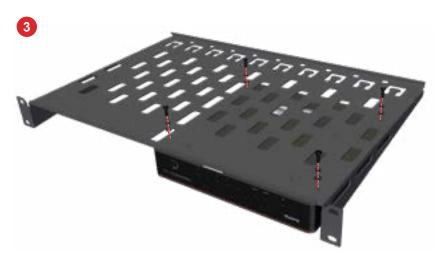
4. Install the rack shelf (hardware provided), and make connections to the devices per their installation guide.
