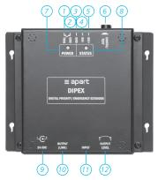
\*When applying an unbalanced line level signal, connector 3 and 4(GND and SIG-) must be shorted using a wire bridge! Connect the ground from the unbalanced source to GND AND SIG-, the + to SIG+. When nothing is connected to SIG-, there will be no sound at all.
