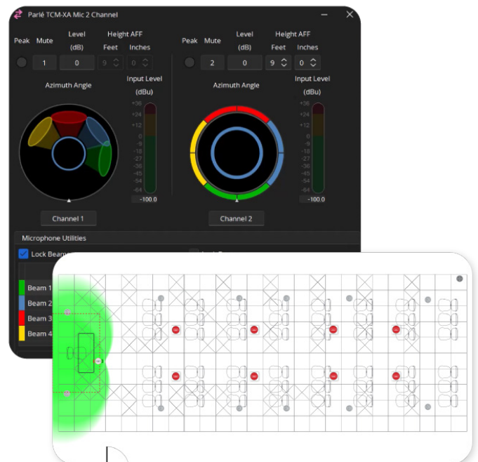
The Parlé Voice Lift interface is accessed through Tesira software.
