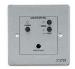
ACPR is a wired remote control with local line input for the SDQ5PIR active speaker. The ACPR audio control panel has a line input at the rear on euroblock connectors and one 3.2 mm stereo jack input on the front panel. This rear line input is in use when no jack is inserted in the front panel jack connector. Inserting a jack automatically disables the rear line input.
