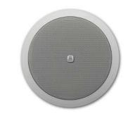
The CM6T is a two-way low impedance or 100 volt loudspeaker suitable for the distribution of microphone calls and background music. In 16 ohms use, you can connect up to 4 loudspeakers in parallel on each channel of a standard 4 ohms amplifier.
