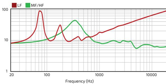
Min Impedance: (LF) 9.3 ohms @ 250Hz, (MF/HF) 5.6 ohms @ 5000 Hz
