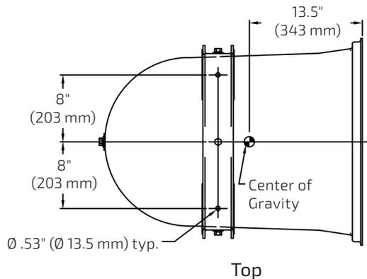
*Note: Cabinets are hand-laminated and measurements vary slightly due to the thickness of the fiberglass. Dimensions shown should not be used to fabricate hanging fixtures. Mounting points are approximate.*
