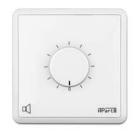
The E-VOLST is a 4 ohms, low impedance stereo volume control that can handle up to 2 x 40 watts of power. It is very versatile thanks to the step-by-step attenuation in 10 steps.
