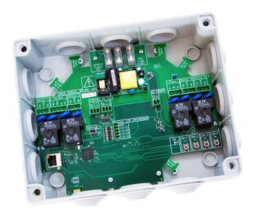
The Impera™ SR-4 is a four-relay unit designed for applications of moderate complexity. Control is via dedicated inputs, one for each relay, accepting control signals from an Impera controller. Separate high-voltage relay connections are provided, as well as a dedicated "screen mode" connection. Test buttons are provided for manual activation of relays, with LEDs for indication of relay state (open or pulled).
