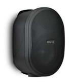
OVO5T is design two-way 100 volt or low impedance cabinet loudspeaker that can be used for background music and paging purposes both indoor and (covered) outdoor. This speaker produces 80 watts @ 16 ohms or when used in 100 volt you can select 30-15-6-3 watts with the easy accessible selection switch at the back.
