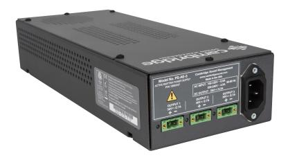
The Active Emitter Power Supply is an external power supply that provides DC power to the Qt® Active Emitter through the Active Emitter Power Injector. It houses three 14/2 conductor cabling outputs that each power up to 50 Qt Active Emitters for a total of 150 Active Emitter maximum. The Active Emitter Power supply is rack or wall mountable.
