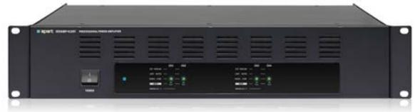
REVAMP4120T is a professional 4-channel digital power amplifier with 4 x 120 watts output power @ 100 volt (or @ 4 ohms), but the unit is also bridgeable to 2 x 240 watts @ 100 volt (or @ 4 ohms). The unit incorporates a high efficient SMPS power supply, outputs with efficient Class D output topology and output transformers.
