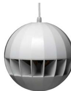
The SPH20 is dual cone 100 volt sphere loudspeaker with a built-in special dispersion cone which gives you a 360° wide dispersion. These speakers allow a loud and wide sound dispersion to be produced with a minimal number of loudspeakers. SPH20 is the most cost-effective solution for background music or speech in installations with high ceilings where you need to cover an expansive area (warehouses, supermarkets, industrial buildings...).
