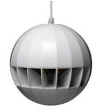
The SPH20 is dual cone 100 volt sphere loudspeaker with a built-in special dispersion cone which gives you a 360° wide dispersion. These speakers allow a loud and wide sound dispersion to be produced with a minimal number of loudspeakers. SPH20 is the most cost-effective solution for background music or speech in installations with high ceilings where you need to cover an expansive area (warehouses, supermarkets, industrial buildings...).
