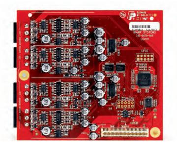
The Tesira<sup>®</sup> EOC-4 is an expander card with 4 analog output channels for use with the Tesira EX-MOD device. The EOC-4 is one of three optional cards that can be mounted in Tesira EX-MOD. Each EOC-4 provides 4 channels of mic or line level audio output. The outputs are electrically balanced and provided on plug-in barrier strip connectors. Software control of each output includes mute, level, signal invert and full-scale output reference.
