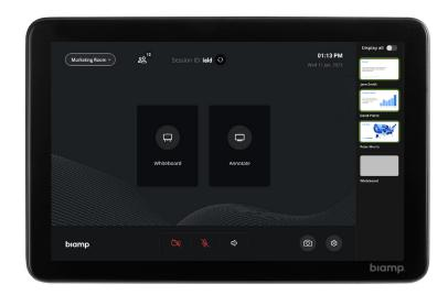
The Touch 8 MAX is an 8-inch, PoE-powered touch panel designed specifically for the MAX Connect BYOM room solution. Using the touch panel, meeting participants can control room peripherals, as well as choose which content to display. Participants can also annotate on shared content and use the digital whiteboard — directly from the touch panel. PIR sensors conveniently turn the touch panel screen on automatically when a user approaches.
