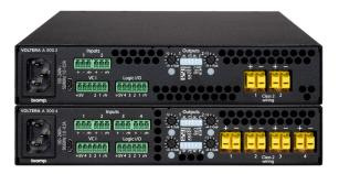
The Voltera® A 300 W amplifiers are half-rack power amplifiers with a total power of 300 W delivered by two or four channels in a sleek, compact design. The amplifier channels are extremely flexible in that they can individually be selected to drive either 4 ohm, 8 ohm, 70 V or 100 V. They also support power sharing so that up to twice the power can be delivered by any channel. Every A Series amplifier ships with mounting accessories for a variety of mounting options.
