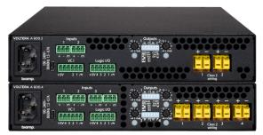
The Voltera® A 600 W amplifier models are half-rack power amplifiers with a total power of 600 W delivered by two or four channels in a sleek, compact design. The amplifier channels are extremely flexible in that they can individually be selected to drive either 4 ohm, 8 ohm, 70 V or 100 V. They also support power sharing so that up to twice the power can be delivered by any channel. Every A Series amplifier ships with mounting accessories for a variety of mounting options.
