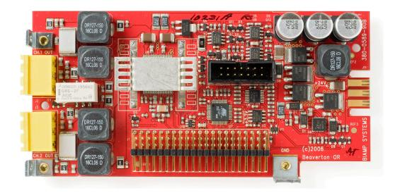
PA-2 amplifier cards allow AudiaFLEX to directly power 4, 6, or 8 ohm speakers. The output power is software configurable from 5 to 30 watts dual-channel and from 10 to 60 watts mono-bridged. An upgraded AudiaFLEX power supply provides a total of 120 watts of power, for up to twelve PA-2 cards.
