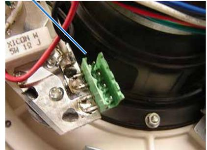
Connect the plug from the can (or from the conduit wiring, see Figure 5) to this socket on the loudspeaker assembly.
