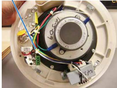
Close-up view of socket for the wiring connector from the back can.
