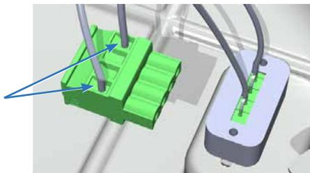
Figure 6. Redeploying the plug for wires entering from conduit
