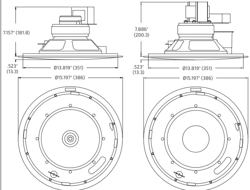
Figure 27. D10 (left) and D10SUB (right) Loudspeaker dimensions
