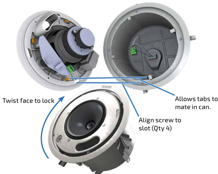
Figure 14. Four *Twist-Assist*<sup>™</sup> face tabs inside the back can instantly secure the loudspeaker to the back can with a twist.
