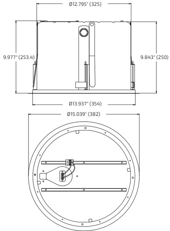
Figure 26. D10 and D10SUB Back can dimensions
