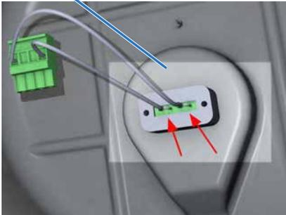
View of 6.5" loudspeaker showing the location of the socket for the wiring connector from the back can.
