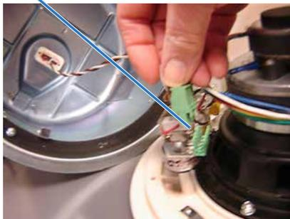
The loudspeaker is now connected to the wires from the can and is ready to mount in the can.
