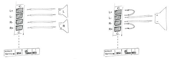
Use at least AWG 18 / 0.75 mm2 speaker cable for cable lengths under 5 meters. Above 5 meters use at least AWG15 / 1.5 mm2. If the speaker manufacturer specifies even thicker cables, follow the recommendation from the speaker manufacturer.
