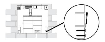
4. Position the speaker template at the speaker-side and mount 3 brackets on the speaker with the short screws.
