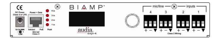
Peak Indicators (Inputs 1–4): These red LEDs will light whenever input channel signal levels exceed 6dB below clipping. Use this feature to aid in the adjustment of the Trim controls (see below).
