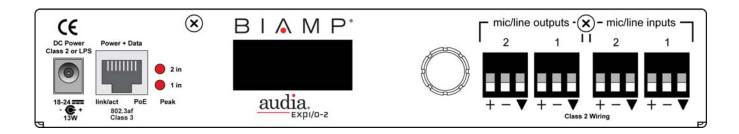
Peak Indicators (Inputs 1–2): These red LEDs will light whenever input channel signal levels exceed 6dB below clipping. Use this feature to aid in the adjustment of the Trim controls (see below).
