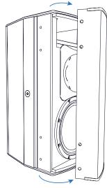
**Figure 3b.** Remove the grille and set aside for reattachment
