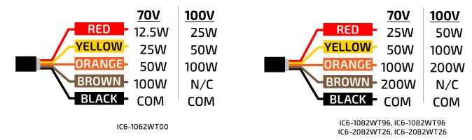
Figure 2. Wiring diagrams for WR/WT (outdoor) models
