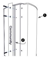
**Figure 7e.** Reinstall the grille one side at a time with correct orientation of the grille retention bars
