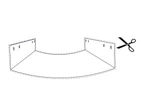
**Figure 7c.** Trim top and bottom of grille cloth, open screw holes, and secure folded sides with glue
