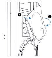
**Figure 3d.** Pull the horn forward and rotate it 90° and realign holes
