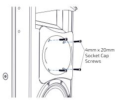
**Figure 3c.** Remove the screws holding the horn in place and set aside
