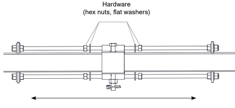
**Step SB-2.** Loosen nuts in the direction the carriage has to go, move carriage to designated position, and tighten hardware
