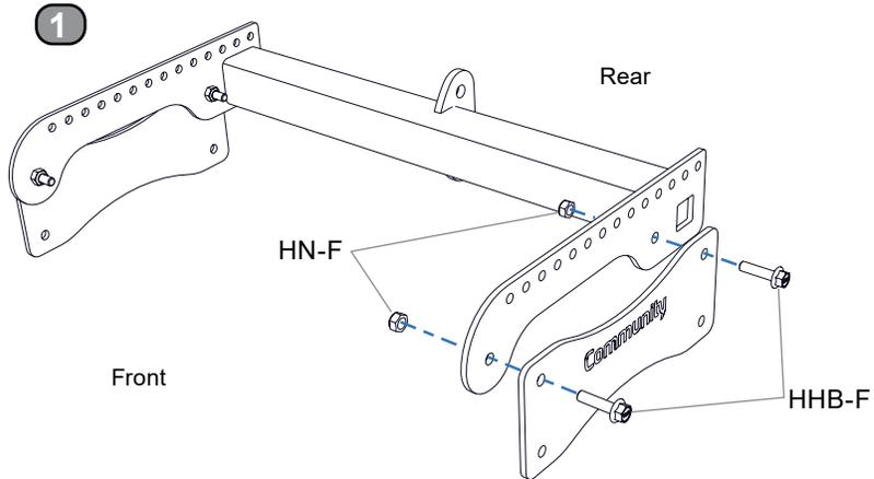
**Step LAF-1.** When used at the top of an array, use the Grade 10.9 hardware, loosely connect the splay brackets to the array frame with "Community" facing out
