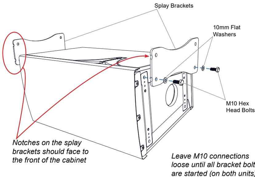
**Figure 1.** Typical splay bracket attachment to a cabinet
