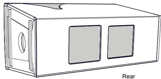
**Figure 32.** Mask off the internal components, threaded inserts, the horn exterior and rear panels
