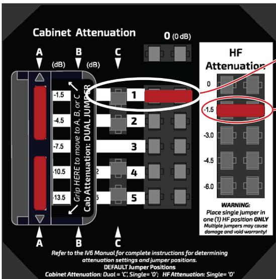
**Figure 24.** Attenuation panel with jumpers set to match VenuePolar cabinet filter setting
