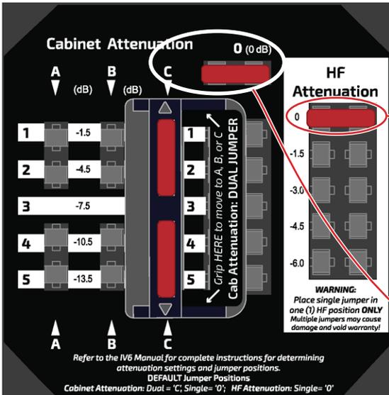
**Figure 23.** Attenuation panel with jumpers set to match EF3 box attenuation setting (Factory default setting)
