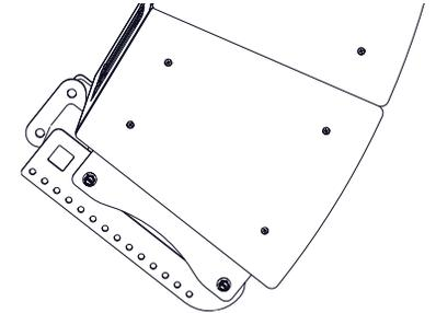
Use as pullback bar at the bottom of a curved array
