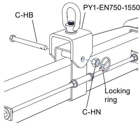
**Step SB-4.** Attach Lift Point to carriage hang point
