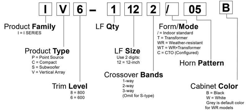
The standard configuration is indoor construction with low impedance operation. All models also have a weather-resistant (WR) option.
