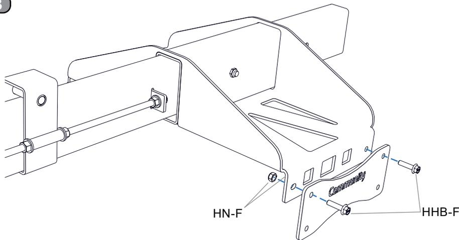
**Step SB-3.** Loosely connect the splay brackets to the array frame
