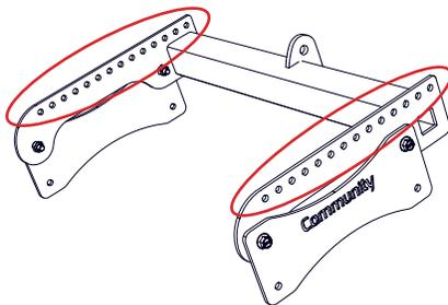
Connect suspension hardware to upper holes along the side rails (circled)
