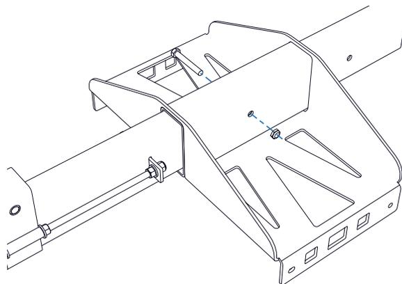
**Step SB-1.** Determine sub mounting position (Reposition frame forward if needed, using installed bolt/nut)
