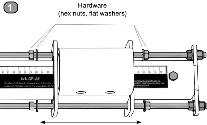
**Step GP-1.** Loosen carriage hardware, move the carriage to suggested pin# position, and re-secure hardware
