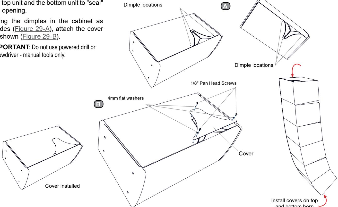
**Figure 29.** Attach covers on each end of the array
