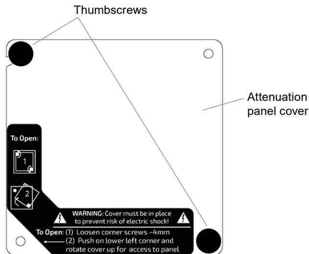
Figure 27. Attenuation panel cover (indoor IV6-1122 models)
