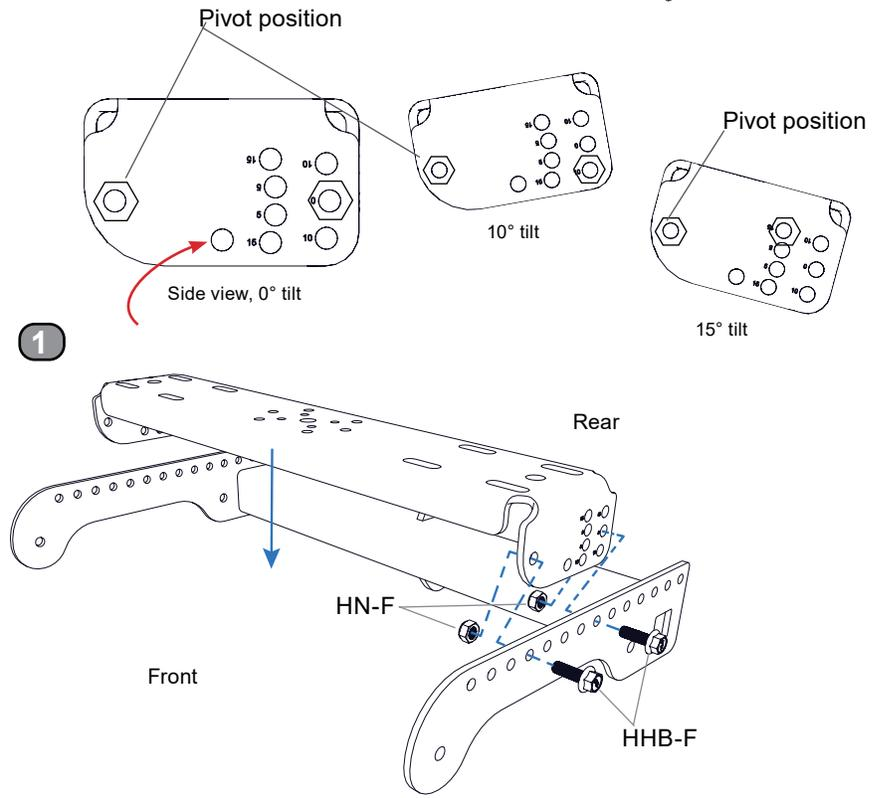
**Step LAU-1.** Attach the U-bracket to the frame at the desired angle, centered around the specified pin point# from EASE® Focus 3
