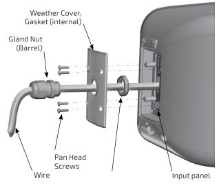
**Figure 6.** Weather cover attachment (*R.15* shown)
