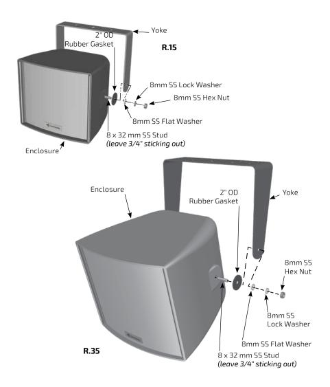
Figure 3. Mount the loudspeaker to the yoke
