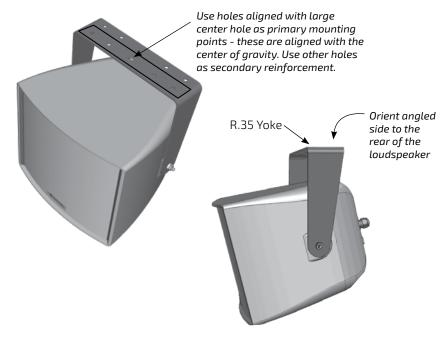
Figure 2b. Orient the R.35 yoke correctly
