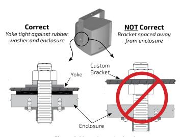
Figure 1. Mounting point load
