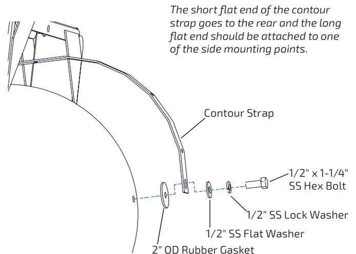
Figure 4b. Attach the contour strap
