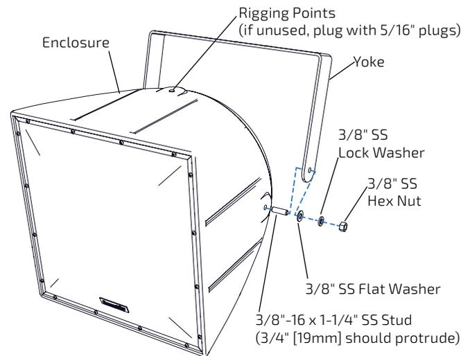
Figure 2. Mount the R.5-MAX loudspeaker to the yoke
