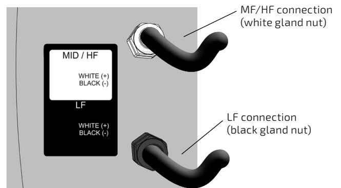
Figure 8. Labeled cables - R2-MAX
