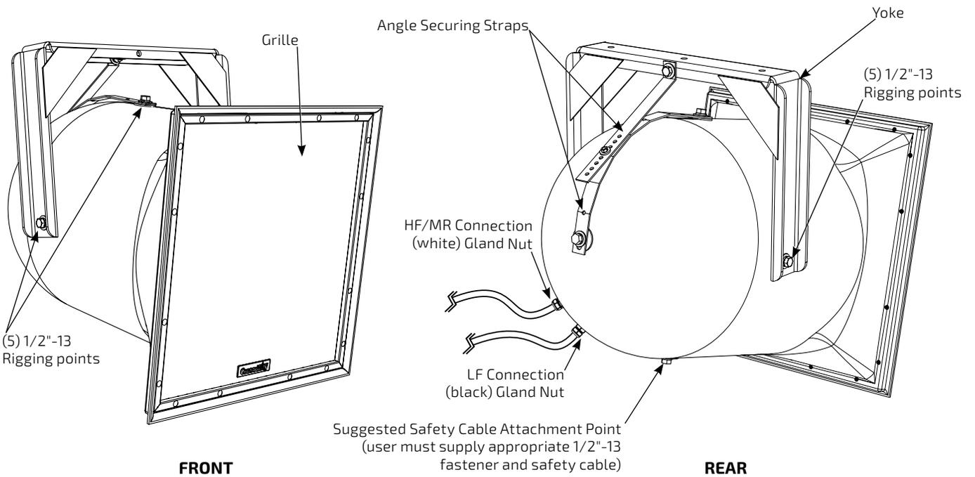
**Note:** Cabinets are handmade and measurements may vary slightly due to the thickness of the fiberglass.
