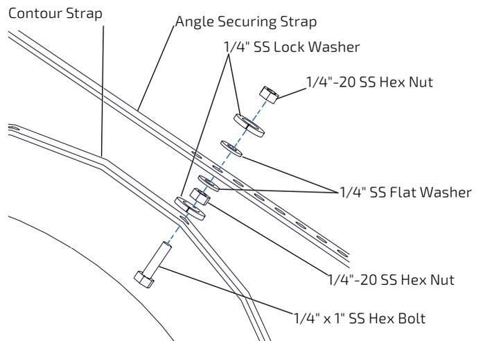
Figure 5c. Attach the securing strap to the contour strap
