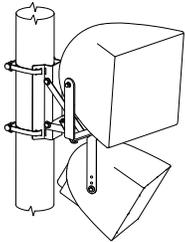
Pole mount bracket kit for mounting one (1) R.15, R.25, R.35, R.5, RMG-200A, W2-218, W2-228, or W2-2W8 loudspeaker, or two (2) loudspeakers in a "top-bottom" configuration, with left-to-right panning capability and vertical downtilt.
