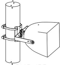
Pole mount bracket kit for mounting a single R.15, R.25, R.35, R.5, RMG-200A, W2-218, W2-228, W2-2W8 loudspeaker. Vertical downtilt to 90°.
