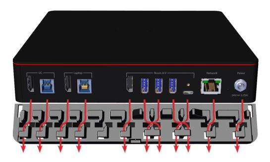
6. Once the device is in a desired location and the cables have been connected and secured within the cable management retainer, attach the protective cover.
