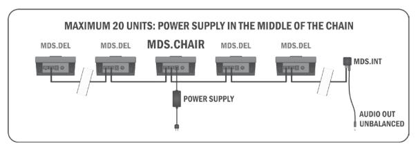
NOTE: maximum 1 chairman unit (MDS.CHAIR) is allowed per system. The unbalanced audio output signal will normally be connected to an amplifier or a pre-amp/mixer.
