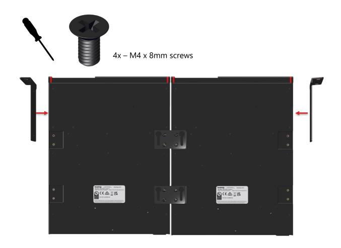
4. Fasten the included device mounting bracket to the left side of the amplifier it came with. Then fasten the included device mounting bracket to the right side of the second amplifier.
