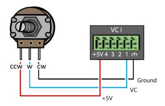
**Note:** Improperly wiring the potentiometer to the Voltera A may cause it to either function in reverse or not function.
