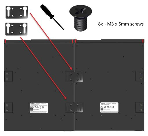
3. Attach 2 of the surface mounting brackets to the bottom of the 2 amplifiers on the surface-mount attachment points where the amplifiers meet. Each bracket should cover the adjoining mount points on both amplifiers.
