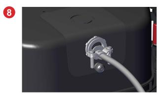
Secure a safety cable to the seismic safety tab. Make the cable as short as possible. Attach the cable to a secondary structural point directly above the seismic safety tab to minimize impact force and swing in the event of a ceiling failure.
