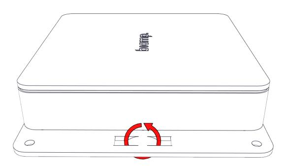
6. Adjust the location of the device as needed before tightening the zip ties enough to secure the device in place.
