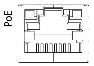
**Port LED indicators:** The yellow LED indicates the link status and the green LED indicates the link speed.
