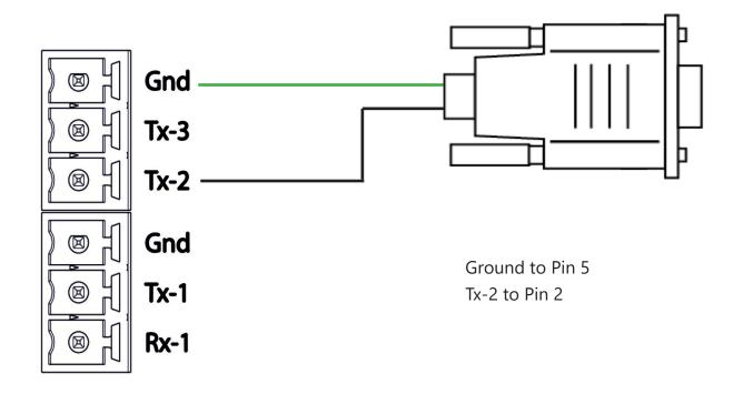
Single IR port unidirectional transmit example.
