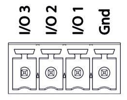
**Potential:** These ports are not potential-free. External relays may be needed to prevent ground loops depending on the application.
