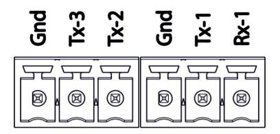
**One-Way Communicatons:** The TX-3 and TX-2 are unidriectional transmit terminals.
