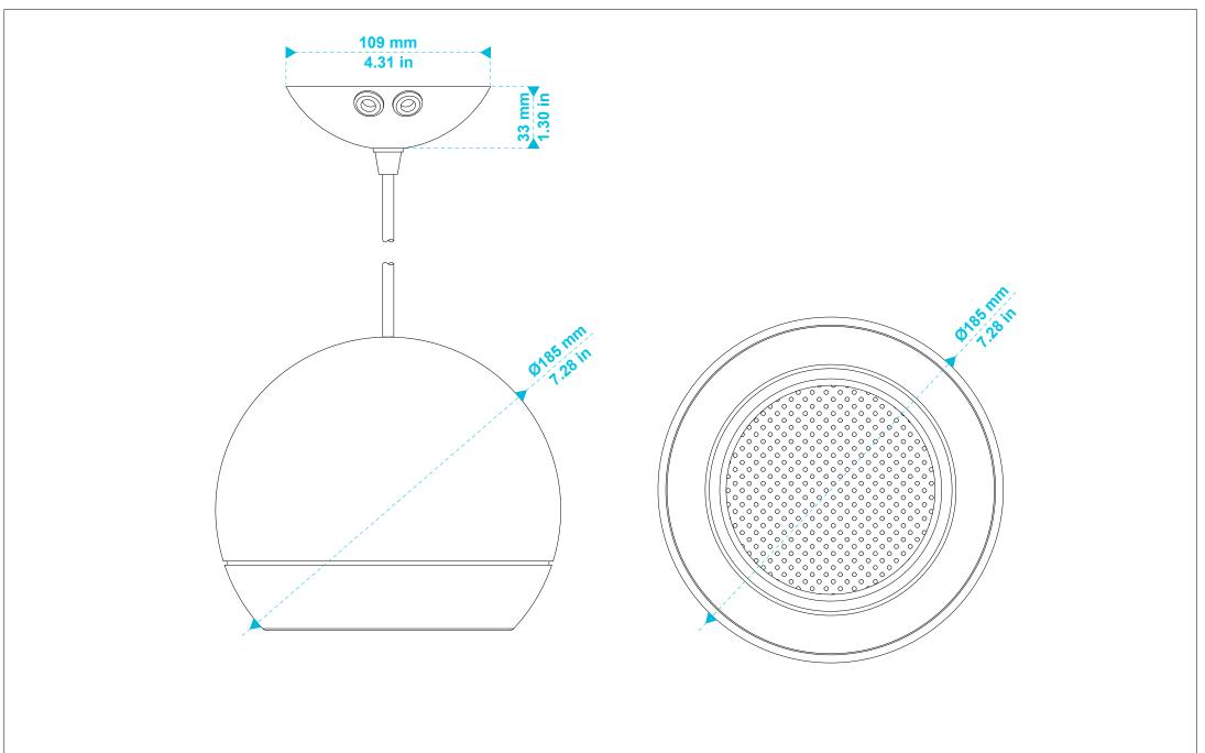
biddebitmodel nameproduct typefile modification dateunit of measurementEN-SPH5T16EN54-24 sphere loudspeaker28th February 2019mm / in
